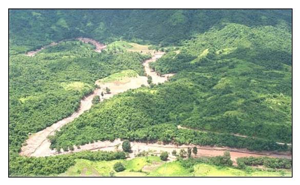
Figure 5-15 Oblique aerial photographs along Nam Ko Yai stream channel. The photograph, at location Z in Figure 5-11, illustrates the flow-flood track along plant debris and soils had been strongly eroded and transported from its banks before reaching the outlet of the Nam Ko Yai sub-catchment.
